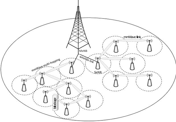
Fig. 1: Illustration of 5G mmWave self-backhaul network.
