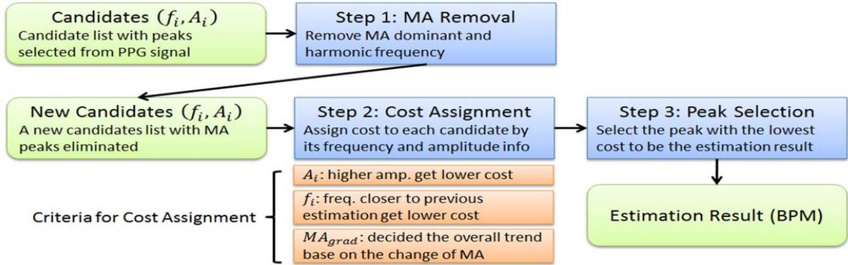
Fig. 4. Flowchart for the proposed peak selection mechanism.
