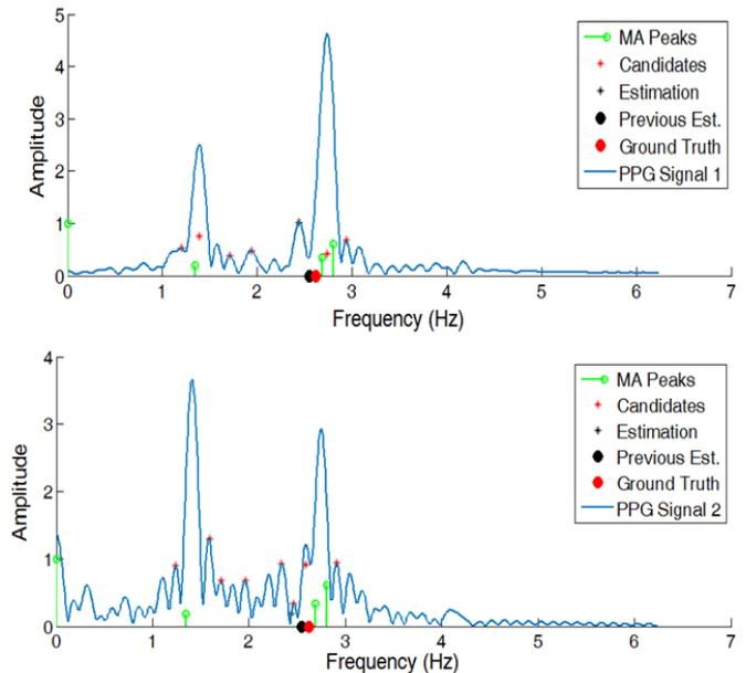
Fig. 10. Special case: The preferred frequency candidate actually has the largest amplitude in PPG signal 1 and the second largest in PPG signal 2. Its location is also close to the previous estimation. However, the preferred candidate has the same frequency as the dominant MA frequency, which makes its cost increased. Therefore, the peak selection mechanism eventually selects the peak near to the previous estimation though its amplitude is far smaller than the preferred one.
