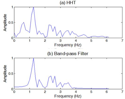
Fig. 2. Signal filtered with (a) the HHT and (b) the band-pass filter.
