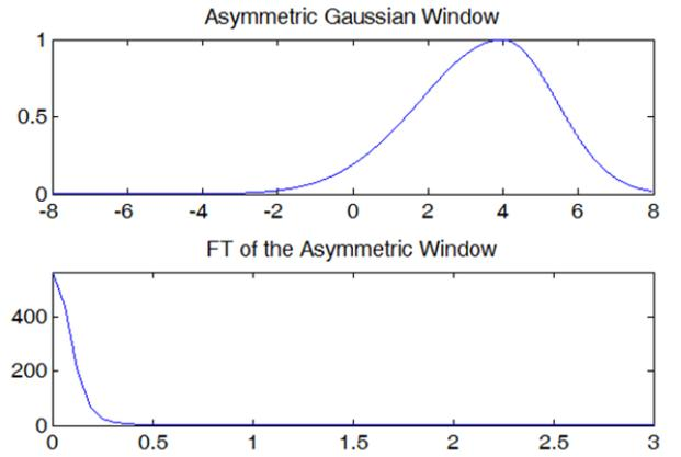
Fig. 3. Asymmetric Gaussian window in (a) the time domain and (b) the frequency domain.
