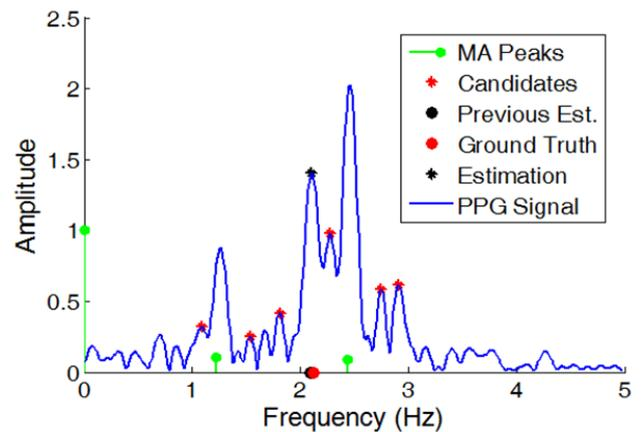
Fig. 9. Frequency spectrum for the 29<sup>th</sup> window of dataset 5.
